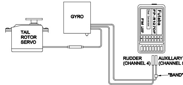
❑ 2. Connect the tail rotor servo to the connector on the gyro (there is only one connector on the gyro that will connect to the servo).
