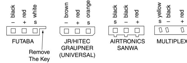
❑ 1. The Heli-Max Mini Piezo Gyro comes with universal connectors that work with all brands of radios. All you have to do is make sure the polarities of your system match the polarities of the gyro connectors. When connecting the gyro to the tail rotor servo and receiver as described in the following steps, refer to the diagram above.
