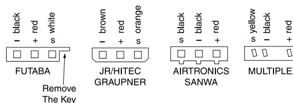
❑ 1. Your Micro Piezo Gyro comes with a Futaba® brand "J" style connector that plugs into your receiver. If you own a Futaba radio control system proceed to step 3. If you own another brand of radio with a different type of connector, you may
