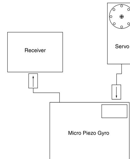
❑ 3. Plug the connector coming from the gyro into the channel in your receiver you intend the gyro to assist (in the case of your helicopter, the rudder/tail rotor channel).
