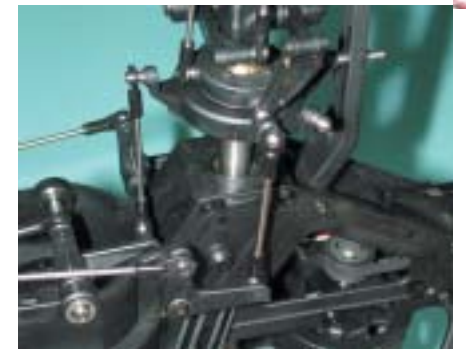
Single servo arrangement with the swashplate rods at 90°.
