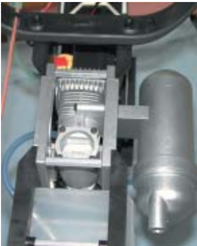
Here we see the engine mount with the pre-installed OS 32. It performed flawlessly, with the correct engine settings being easy to achieve and retained all the way down to the very last drop of fuel!
