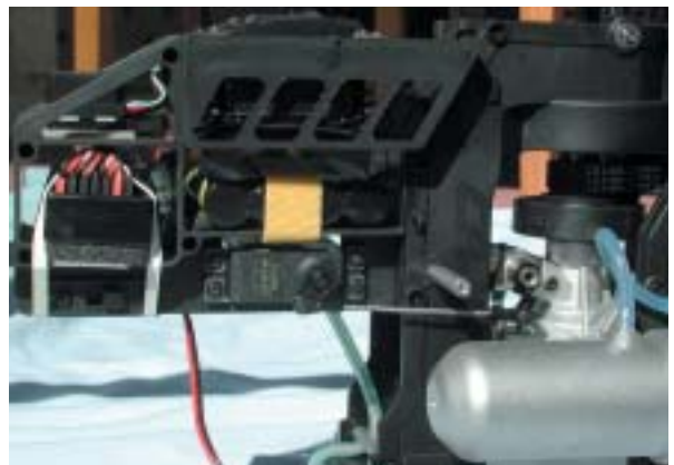
Throttle servo is perfectly sited, note the neat radio installation. The spartan cooling duct has proved perfectly adequate with no signs of overheating.
