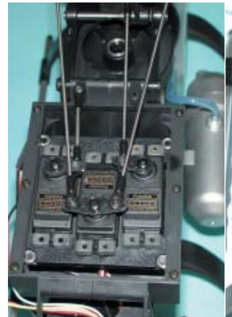
The single-servo control system uses a sliding tray system where the collective servo slides the tray back and forth. The tray is ball raced and may need some shimming and bracing to eliminate play.
