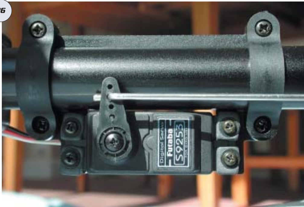
No need for upgrades here, as the 'rear tail rotor servo mount' is supplied with the Caliber 30, thus ensuring accurate friction free control to the tail end. The 'Z' bend may be replaced with a ball link if wear develops.
