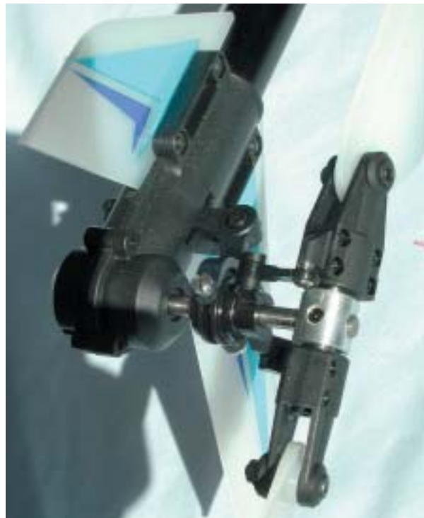
Accurate tail pitch control is achieved via this well thought out 'dual control support system'. Also note how the tail fin in centre mounted and the pitch lever runs through the centre of the boom.
