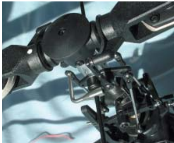
Here we see the heart of the Caliber's sweet and very progressive cyclic response. The rotor head consists of a GRP rotor head yoke with substantial aluminium supporting centre hub. In 'training mode' blade grip is flipped over to trailing edge input and the pitch ball on the lever is relocated to the other side of the pivot point.
