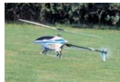
A fully driven tail rotor ensures total control over the tail end in power off Autorotations scenarios like this one.
