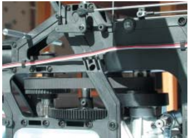
Here you can see the belt primary drive with secondary gear reduction. The auto unit is on the lay shaft providing constant tail drive. Note the neat servo lead clips.
