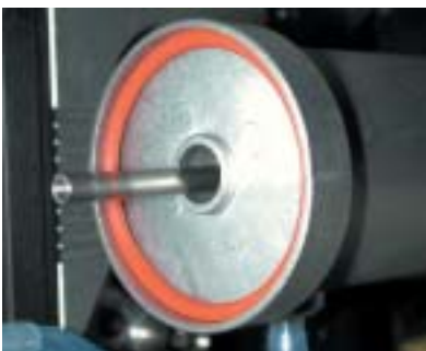
The rear chamber of the kit muffler is sealed with an 'O' ring. The muffler certainly helped the Caliber 30 to retain its whisper like qualities regardless of main rotor speed.
