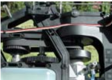
The two-stage belt driven gear reduction system results in a very smooth running gear train and the model also features a constant driven tail rotor for full directional control in auto-rotations.
