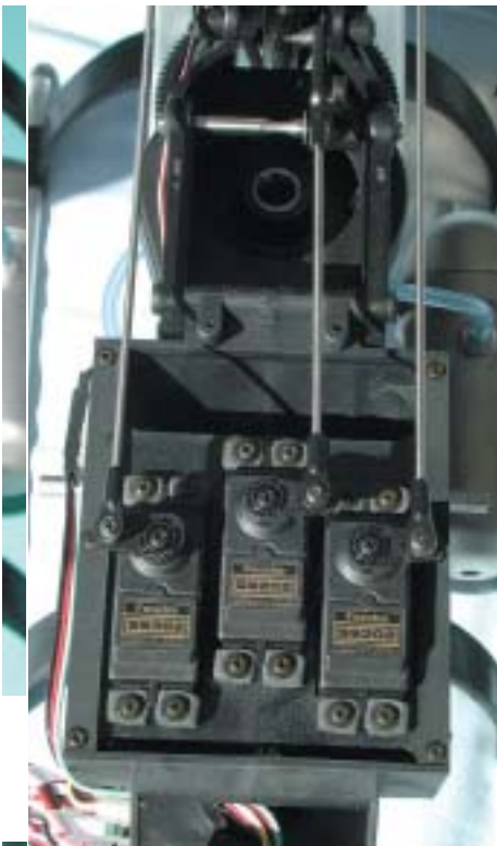
eCCPM servo use a fixed mount in the servo compartment.
