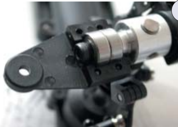
At the tail end, each tail blade grip is supported by two ball races, with a substantial metal tail rotor hub to ensure accurate control and a long service life.
