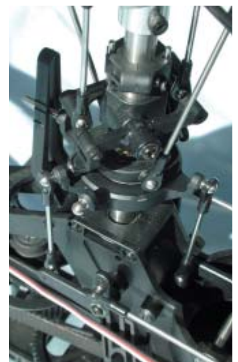
Here, 120° eCCPM is used, note that the bellcranks have been relocated and the input ball is moved to compensate for the reduced servo movement with eCCPM.
